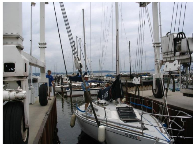
After engine problems, Bretwalda was lifted from the water (at angle to keep fuel in one corner) in Muskegon for repairs
